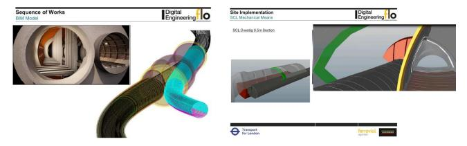
Images of the Step Plate Junction and the tunnel over-dig
